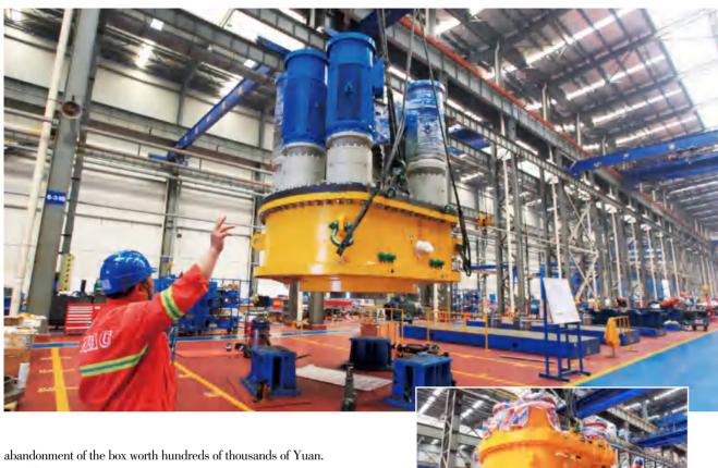
"It requires the processing meeting the requirements and avoiding accidents in the processing as well, including broken cutter and deformation of round holes." When mentioning such a large pieces of 4m in the diameter and 2m height after closure, totally more than 30t, Zhou Jun, Manager of box processing workshop was still somewhat fearful.
