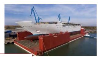
The cruise is 323.6m long totally, with maximum width of 37.2m, height of 72.2m, maximum draught of 8.55m and maximum speed of 22.6n mile/h.
