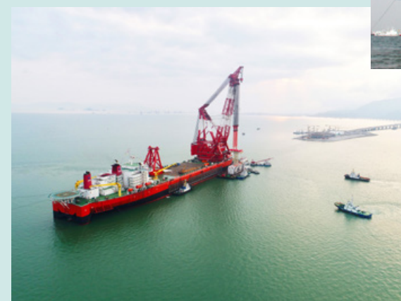
12,000t floating crane Zhenhua No. 30 lifting final joints.
