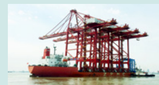
Zhenhua No. 32 with commercial power receiver, loaded with STSs, leaving terminal of Changxing Base.
