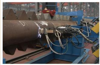
窗户板全位置窄间隙生产线自动焊接 Window plate full-position narrow gap auto welding production line
